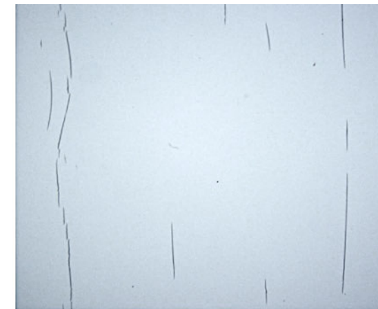
PVDF Cracking after 84 days phase 1 + 42 days phase 2
