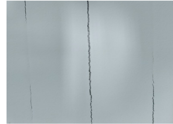
PA Cracking after 120 days in Phase 1
