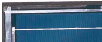
Silicone encapsulant delamination
