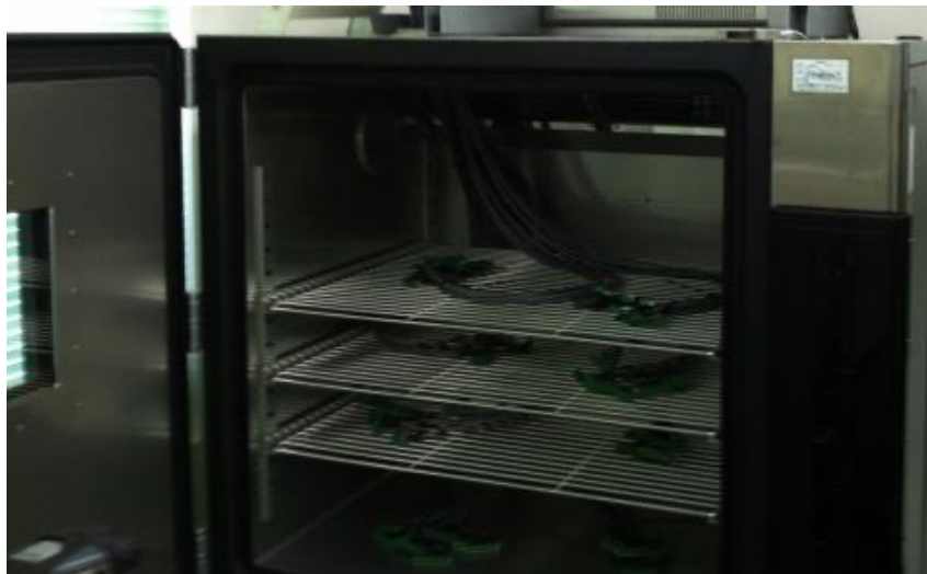
Damp heat chamber for aging samples
