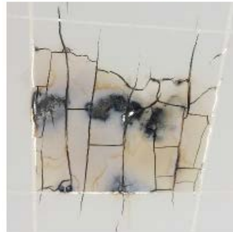
Cracked cell with multiple hot spots
