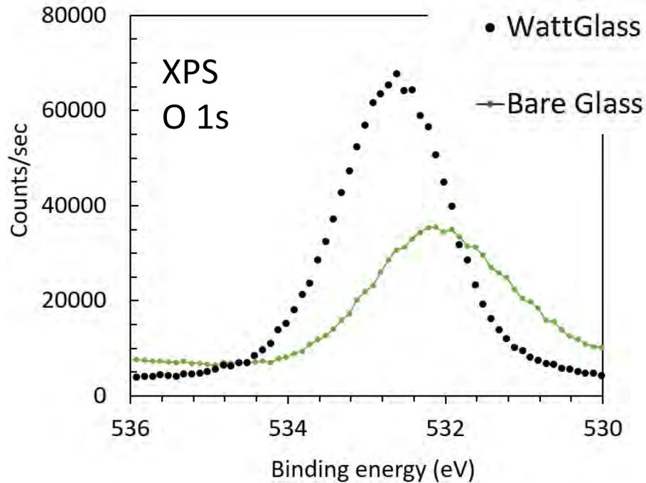
Coating is easily differentiated from bare glass by both techniques
