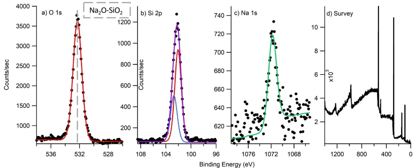
**Hypothesis:** Sodium Silicate ( $\text{Na}_2\text{O-SiO}_2$ ) is forming at gridlines
