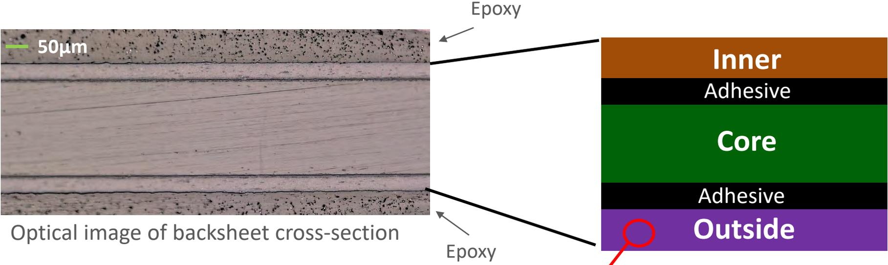
Optical image of backsheet cross-section
