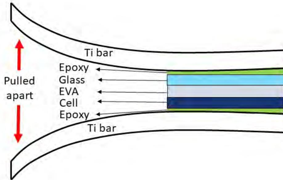
Debonding energy of encapsulant/metalization interface drops off when exposed to damp heat and/or high voltage
