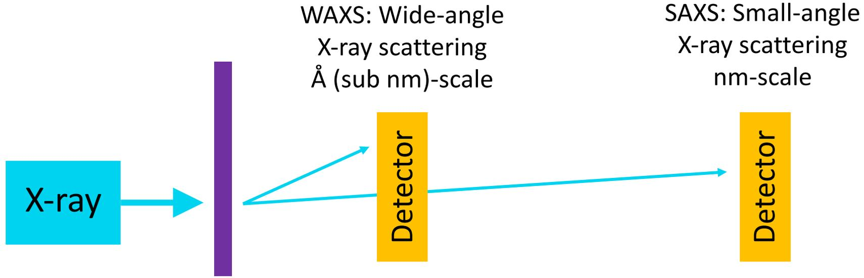
X-rays scatter off of differences in electron density
