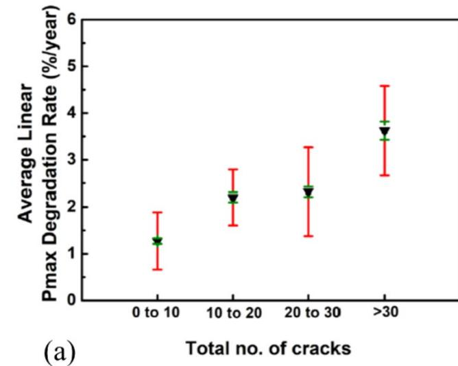
(a) Relation of degradation rate and crack number
