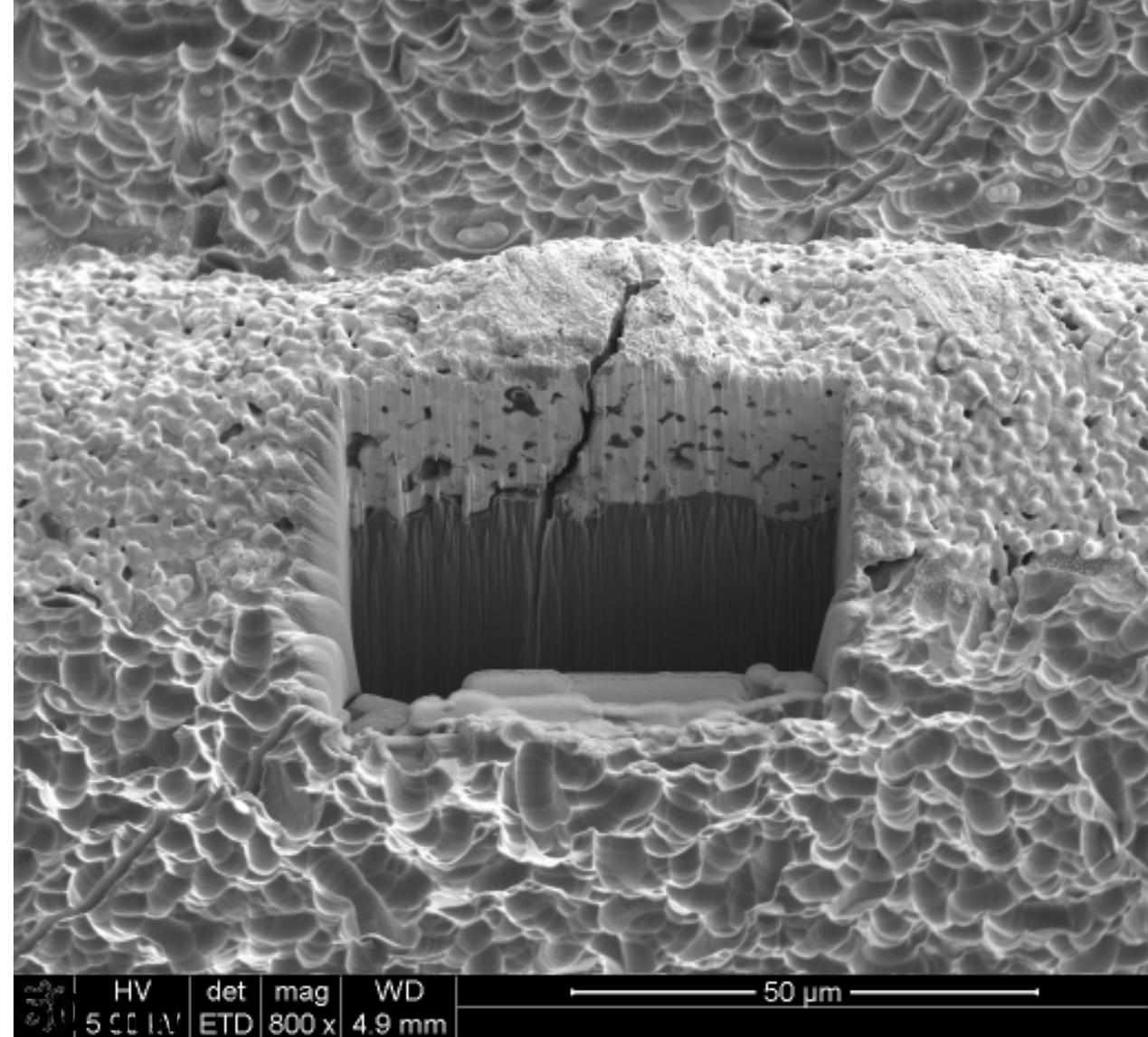
Broken metallization creates rough contact
