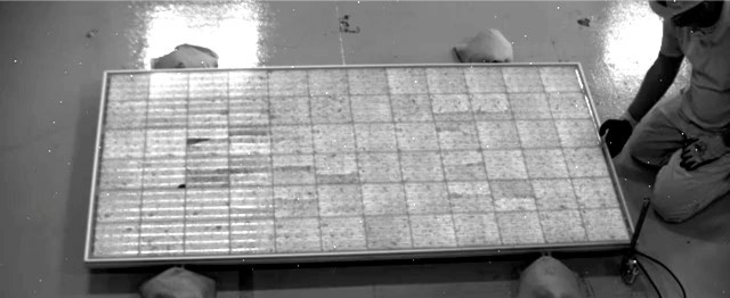
We tested commercial 72-cell mc-Si modules
