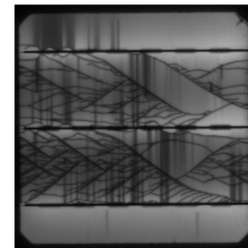
Electroluminescence image of cracked cell<sup>1</sup>
