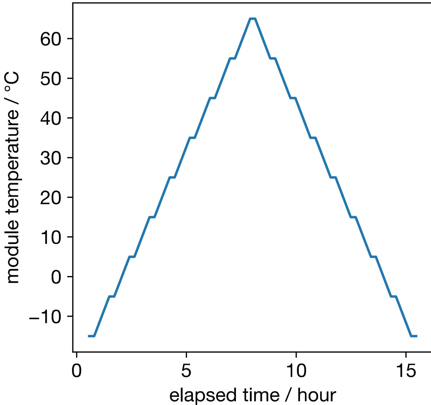
We collect EL images at a 'staircase' of temperatures
