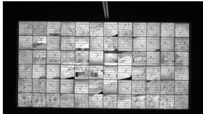
Electroluminescence image of solar module in lab
