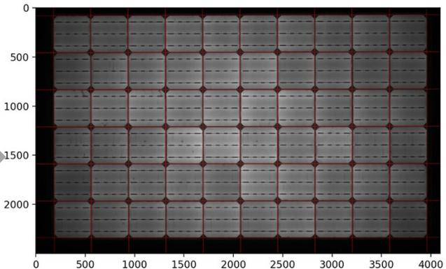
Detected internal edges from the whole module
