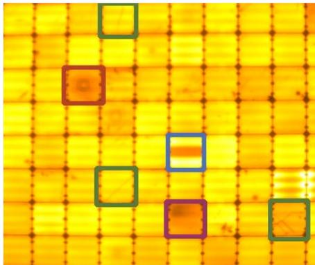
Electroluminescence image of solar module in field (defective cells are labelled with box)
