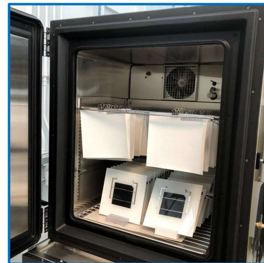
Coupon and MiMo specimens in hygrometric chamber
