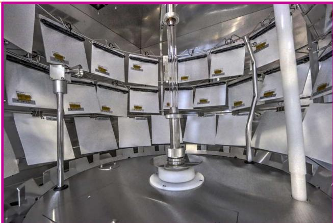
Coupon and MiMo specimens in Xe UV chamber (inside the carousel)
