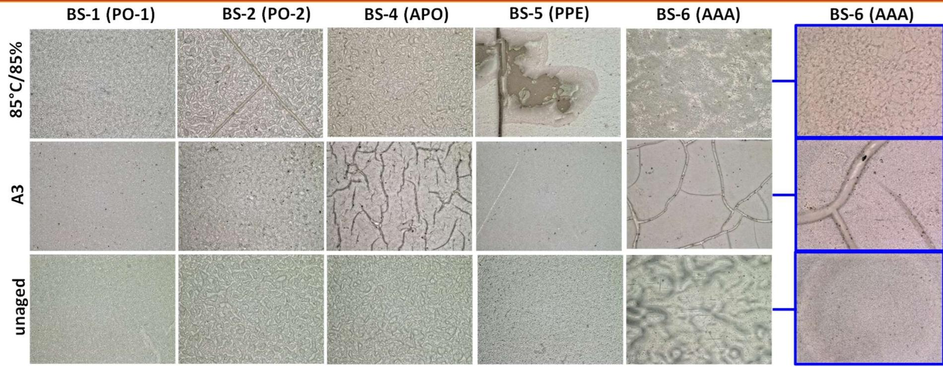
Comparison of surface morphology at 4000h (85°C/85% RH and A3) relative to unaged.
