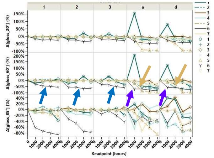
Comparison of  $\Delta$ [gloss] at coupon center for air side BS's through initial 5 experiments.
