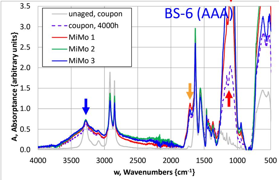
FTIR spectra for A2 UV weathering.
