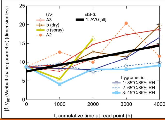
Breakdown voltage ( $\alpha$ , scale parameter) and variability ( $\beta$ , shape parameter) of BS-6 through the most affecting of first 5 experiments.
