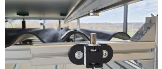
Contactless displacement sensors mounted on framing and modules
