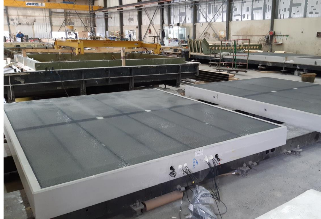
Road elements are monitored real-time using thermo-mechanical packaging to study the load of passing vehicles
