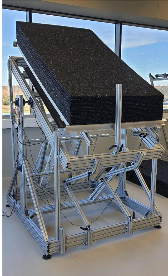
Mechanical load performed test at 30° angle
