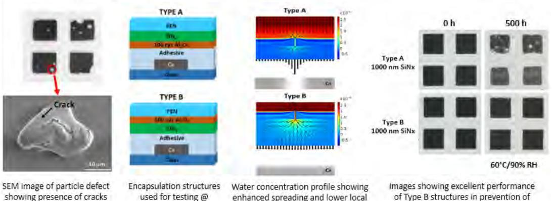
showing presence of cracks in the vicinity of a particle
