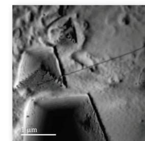
TEM example of a dislocation in a silicon solar cell
