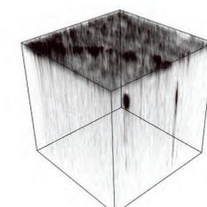
3D Render of Na+ Measured area: 200 x 200 x 3.5µm
