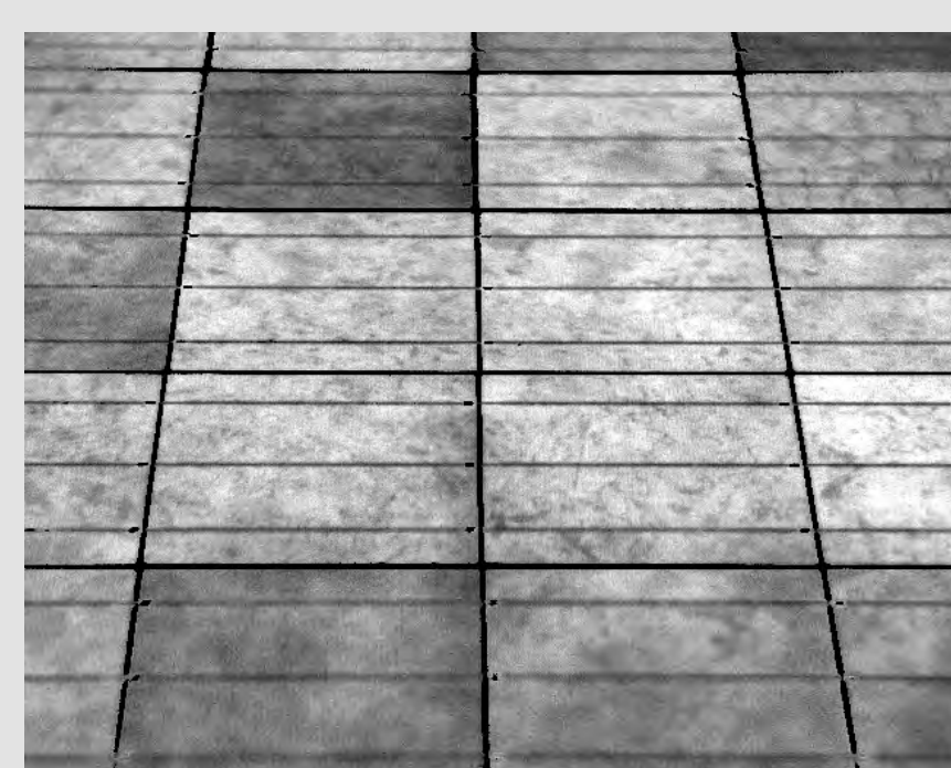
Outdoor PL imaging of c-Si in full sunlight
