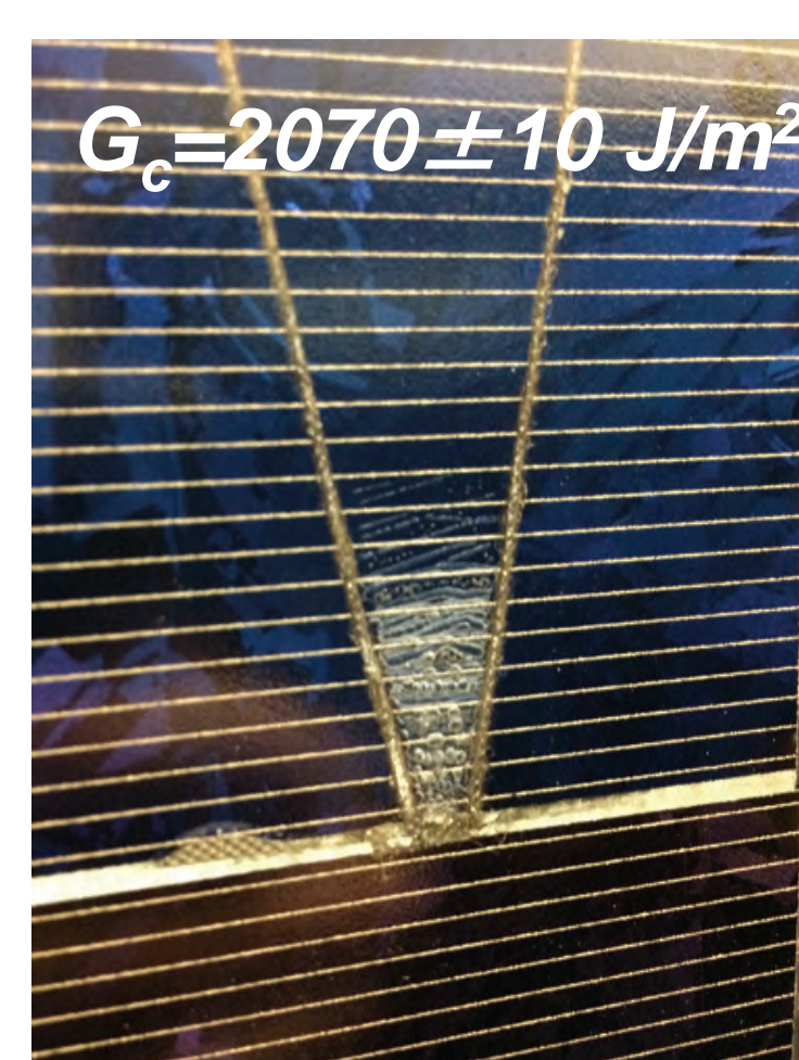
BP module deployed 11-years in Ohio with no delamination
