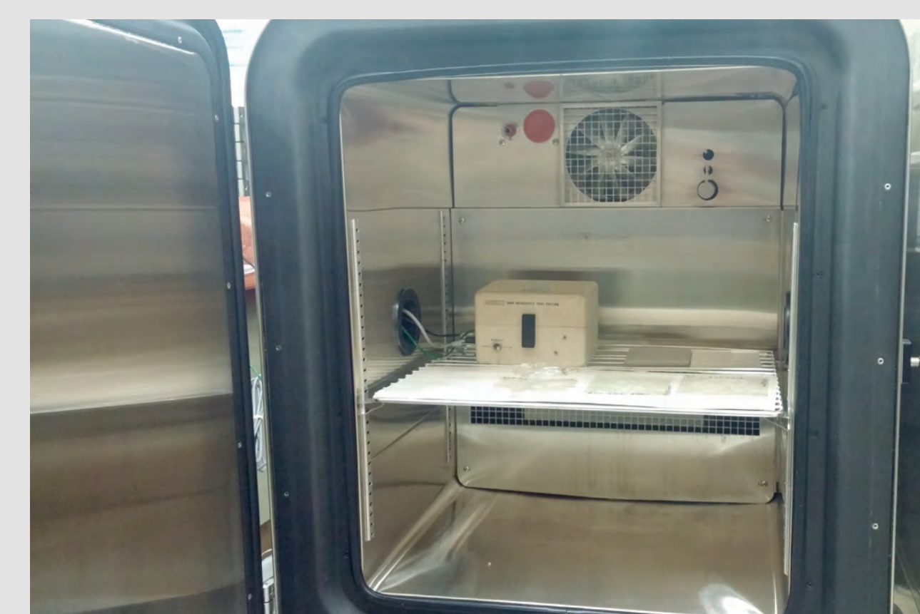
Resistivity measuring equipment placed in a humidity chamber to enable measurement of resistivity at controlled heat and humidity.
