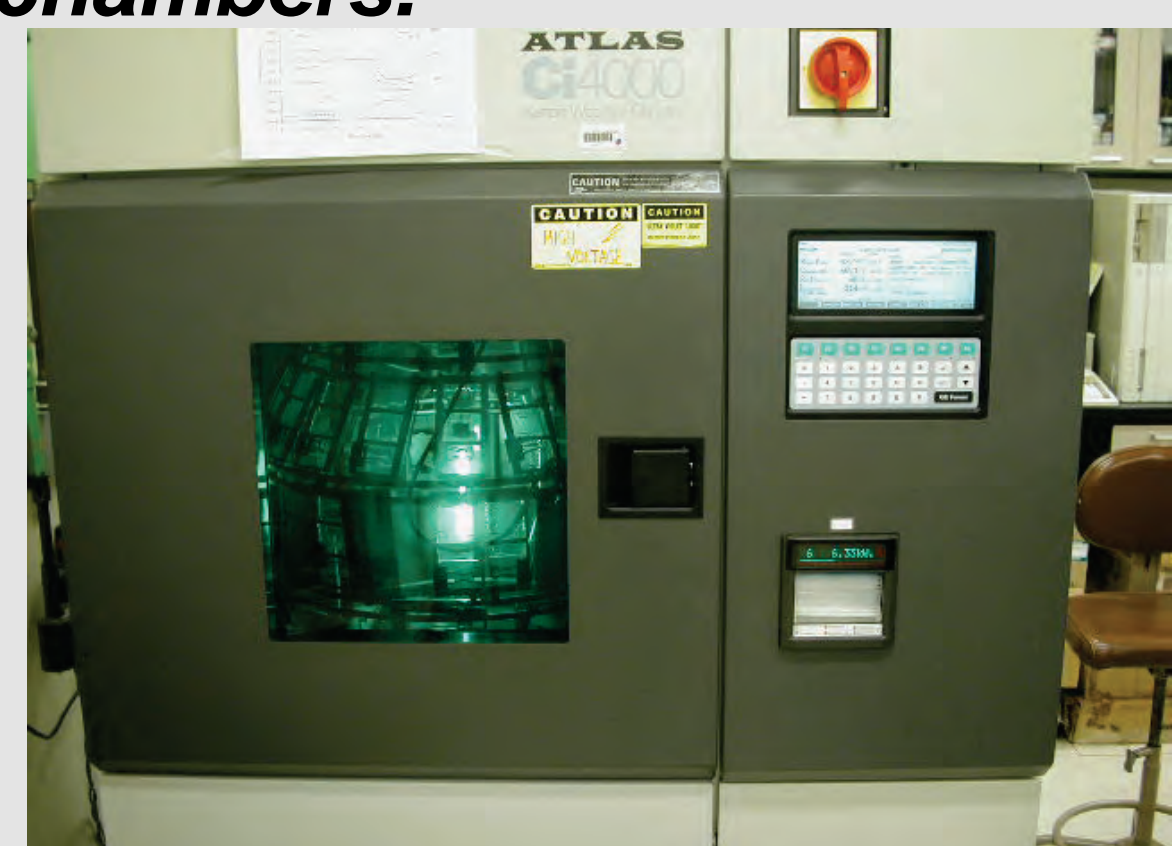
One of many Weather-Ometers capable of exposing samples to controlled irradiance, temperature and Humidity.
