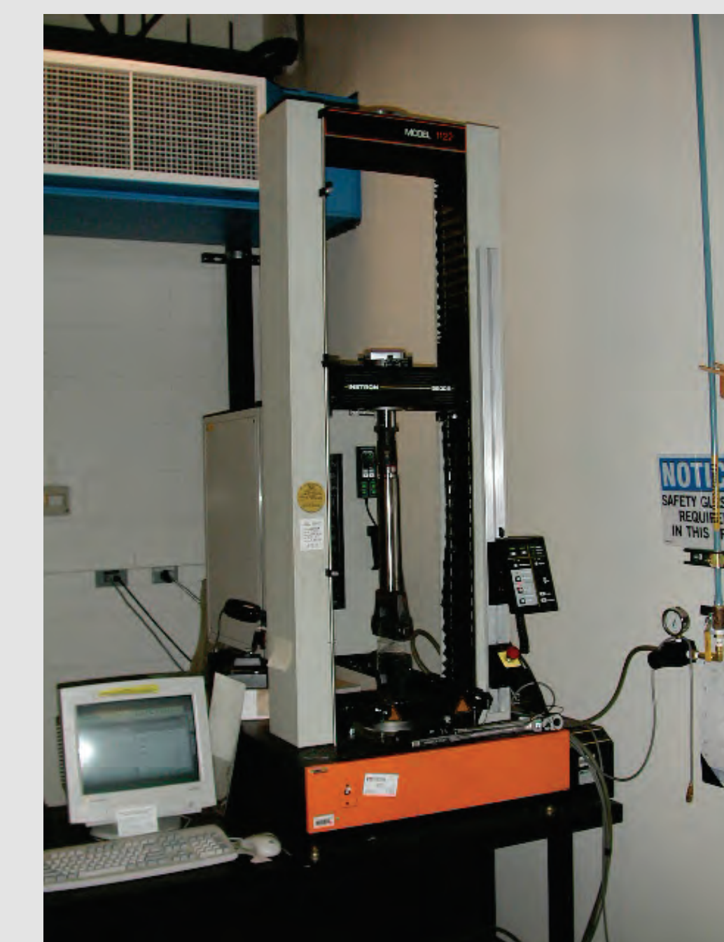
Instron puller for measuring adhesion or mechanical properties of materials.
