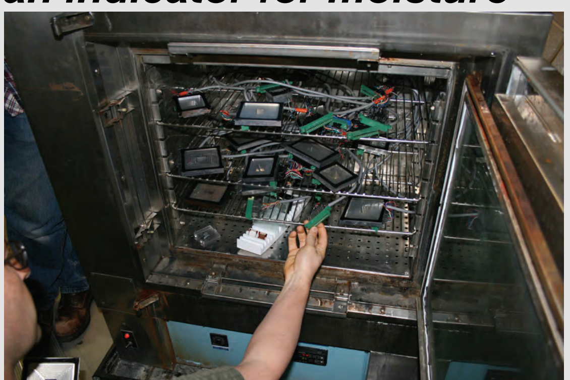
Chamber equipped for simultaneous measurement of up to 32 films at once.
