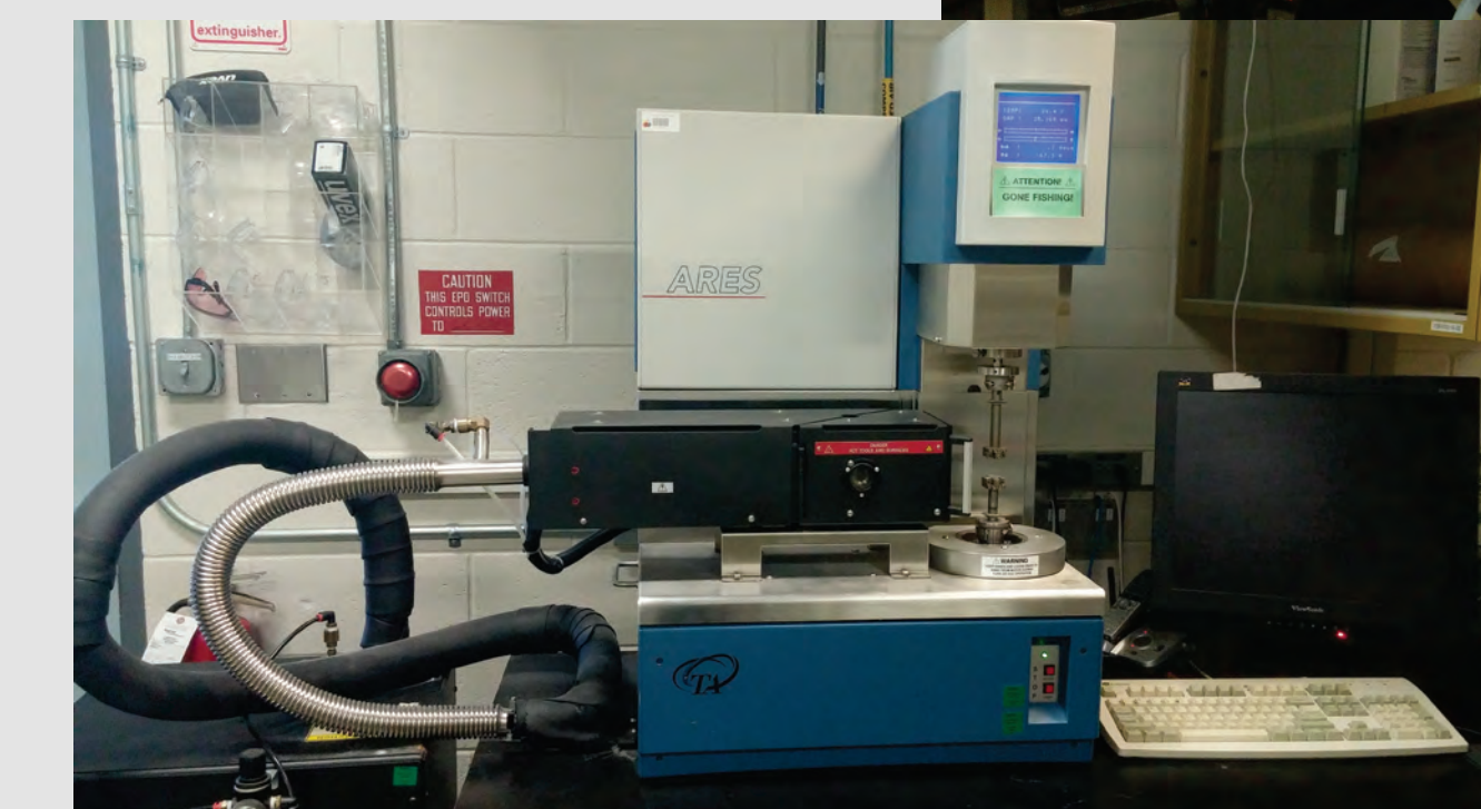
TA Instruments rheometer used for measuring the mechanical moduli of PV materials.
