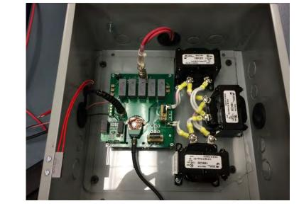
High-power test system for evaluation of power semiconductor switches
