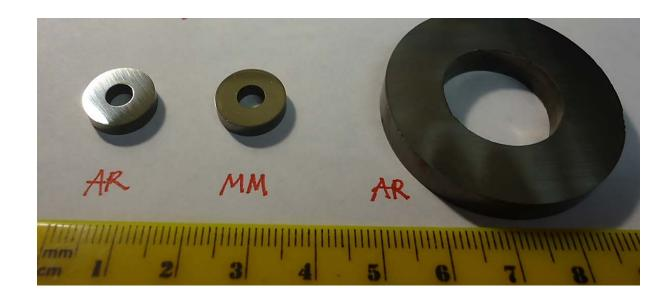
Net-shaped and sintered toroids (no machining required)
