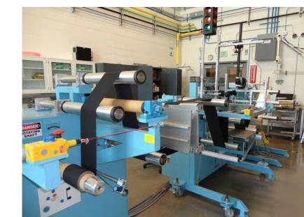
High speed roll handling equipment for in-line inspection & metrology development as well as potential for expansion for processing
