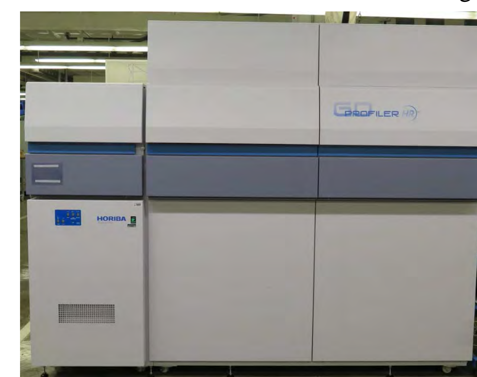
GD Profiler HR, Measure the oxidation and diffusion of materials during aging and degradation process in the depth direction
