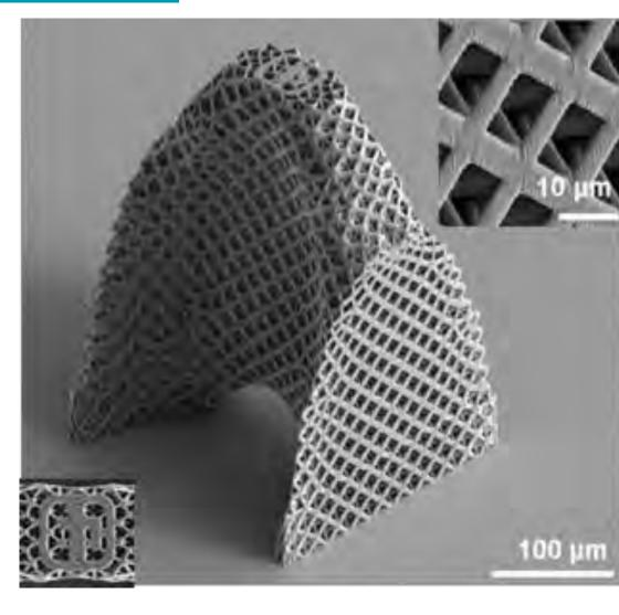
Additive manufacturing technologies support rapid component realization
