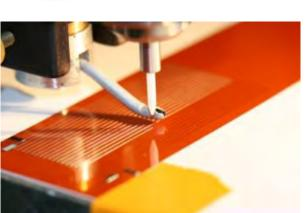
Direct write technologies enable access to materials not supported by conventional printing processes
