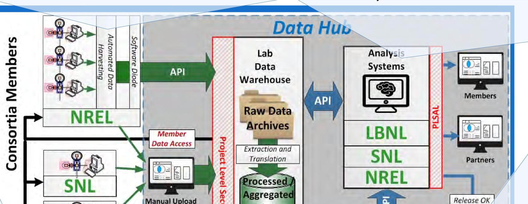
In order to move data into the archives, those labs where automatic harvesting can be performed will utilize an API connection. Others can transfer data manually through the web site templates. The templates will be built on data standards and a common format that we will need to establish in order to capture a complete representation of the process that went into the sample measurement, synthesis or the parameters defined for the generation of analysis, modeling, or simulation data.
